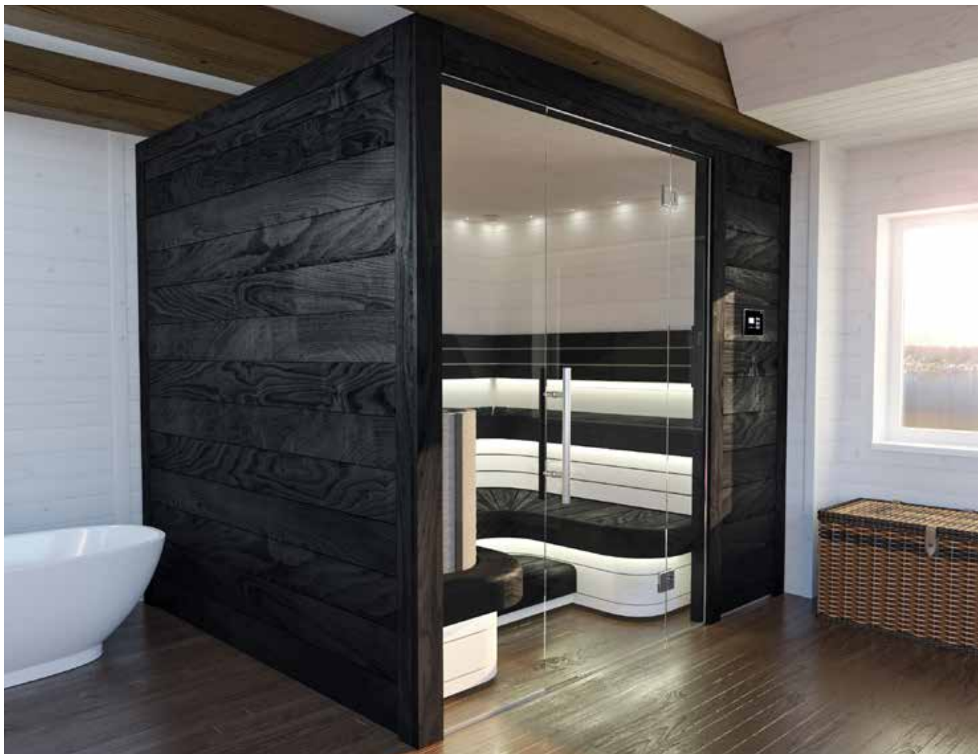
A stylish black-and-white sauna made with painted natural radiata pine panels – walls STS4 19 x 185 mm and benches SHP 26 x 90 mm and 26 x 140 mm. PRIVATE SAUNA, FINLAND
